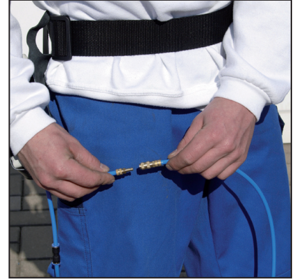
Connect the hose from the telescopic pole to the control unit (Gold coloured connection)
