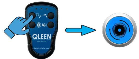
3. Switch off the remote control with the power switch to »0«
